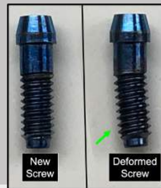
Figure 2: Abutment screw deformation (green arrow) from repeated removal / insertions in comparison to a new screw.
